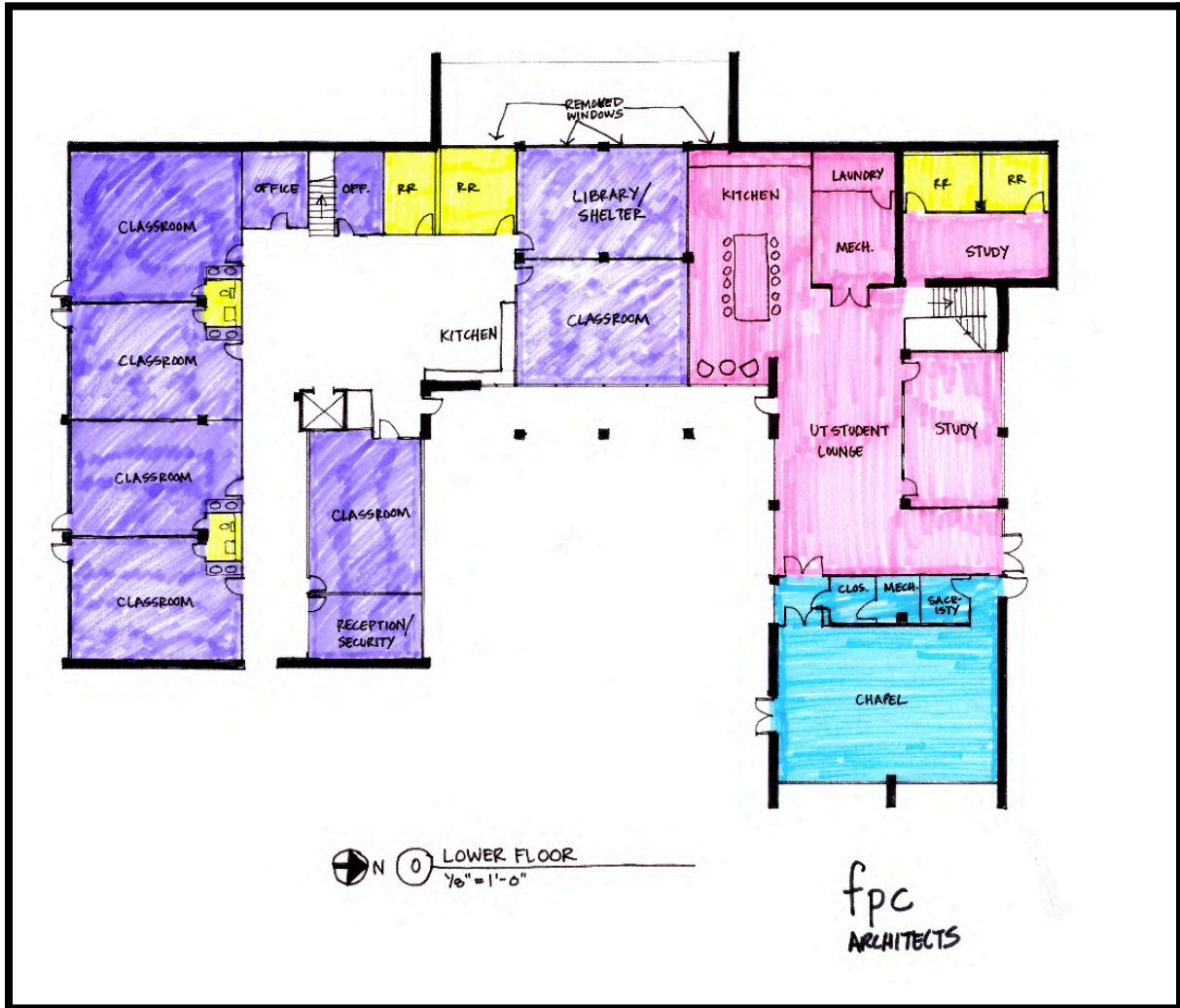
Figure 24. Team #3's proposed lower floor of Gregg House, accommodating Day School expansion and a consolidated Student Center by removing the eating area that is currently between the two anchor tenants. In this proposed plan, the Day School would include a reception/security room at the current entrance, adult restrooms, a new classroom, a large central gathering and eating area served by an L-shaped kitchen, and a windowless library/shelter/safety room.
