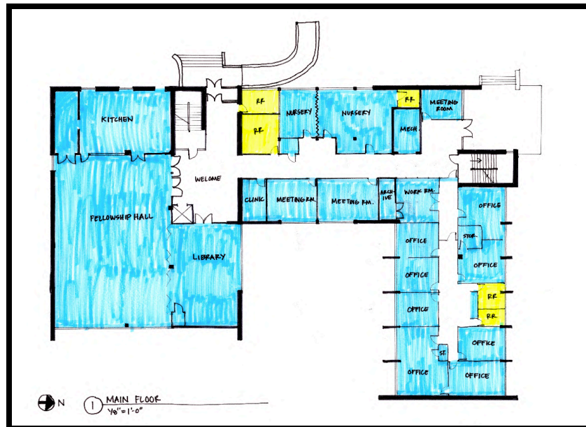
Figure 23. Team #3's proposed main floor of Gregg House, including an elevator adjacent to the Fellowship Hall, a health clinic, and meeting spaces in place of the choir room. Overall, Team #3's approach involved redistributing spaces without changing the building footprint.
